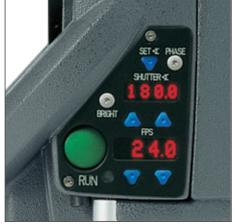
ARRICAM Lite Extended camera control panel
