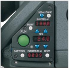
ARRICAM Studio: Extended camera control panel
